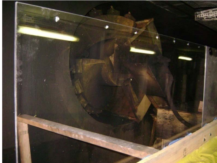
Figure 22: View of headgate cutting drum through partial barrier
